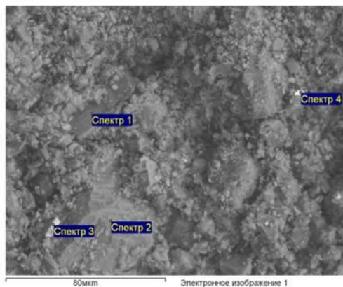
Figure 1 - The microstructure of loess loam from Chaganskiy deposit indicating the point locations of analysis of the chemical elemental composition
